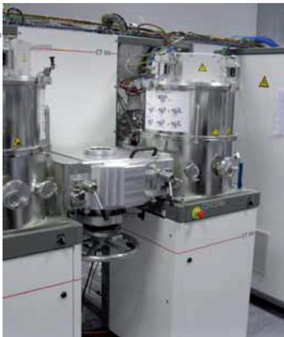
*Sputtering systems at the Catalonia Institute for Energy Research (IREC) for the development of back contacts and transparent conductive oxide (TCO) layers.*
